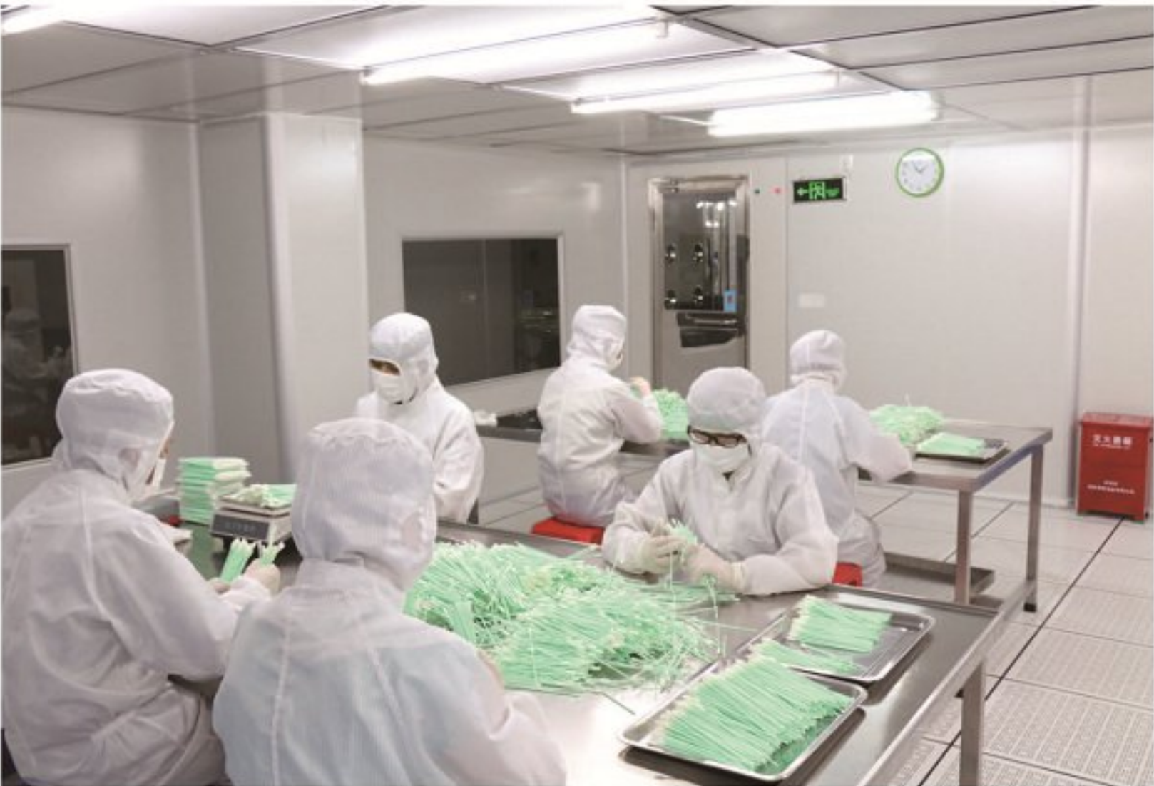
Cleanroom Swabs Final Inspection & Packing Process
