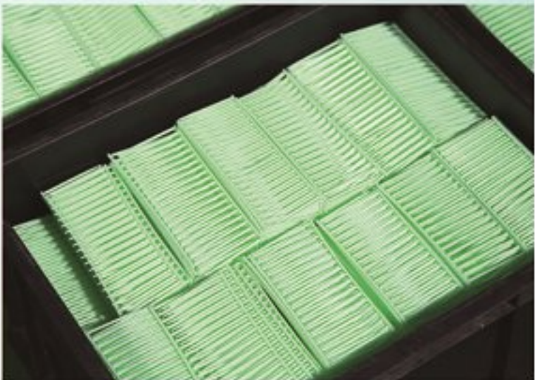
In-House Injection Molding Process for Swab Handle ( Inspected Molded Handle )
