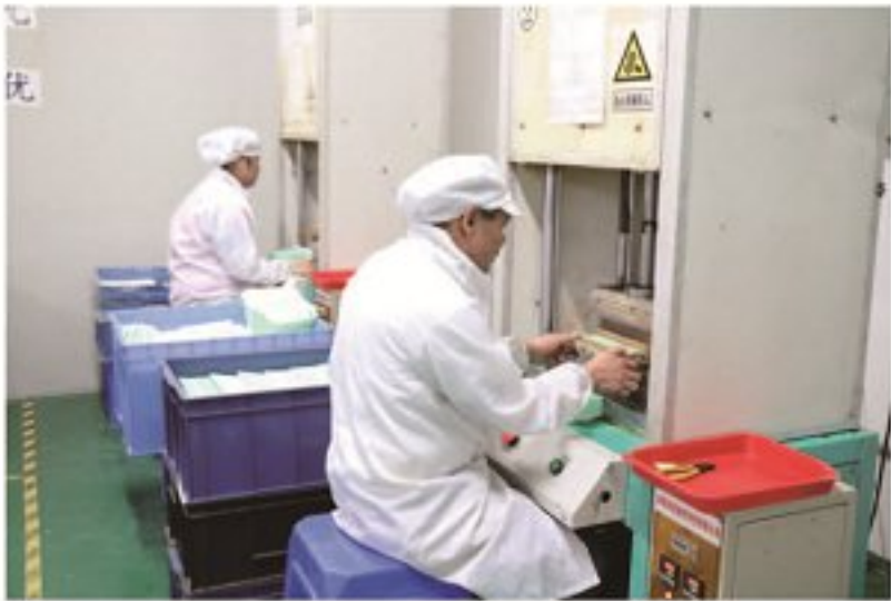
Swab Head Forming Process ( For Foam and Fabric Tip )
