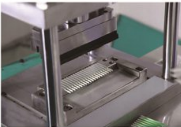
Swab Handle Final Cutting Process ( After Passing Inspection on Swab Head Quality Checking )
